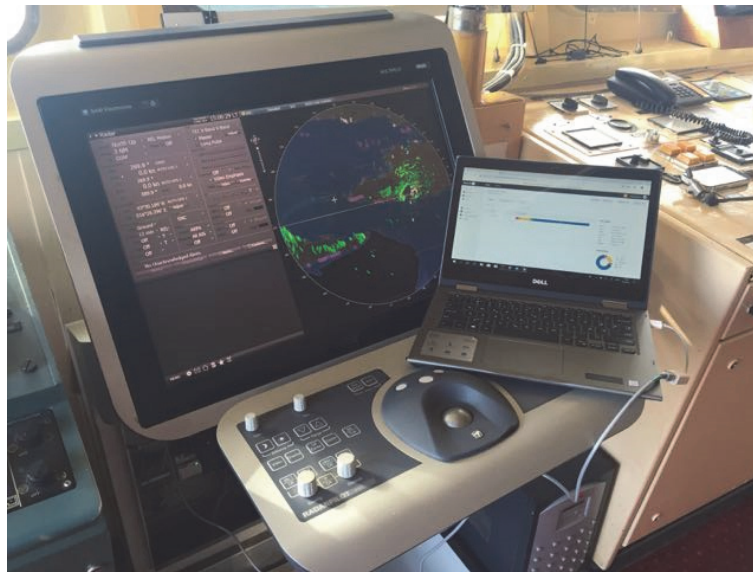
Figure 2. Cyber security testing of the chart-radar.
